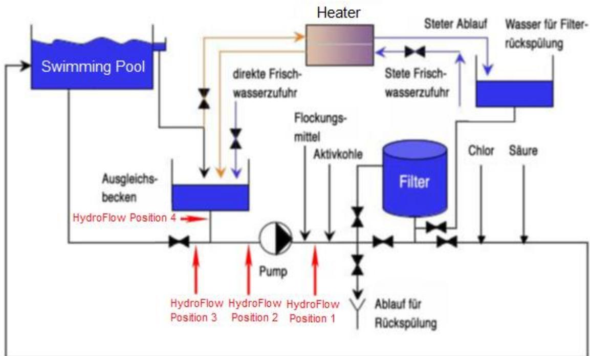
By using the AquaKLEAR device, flocculent dose could be reduced to one-tenth and take the active carbon filter out of order. This extended the backwash interval of the sand filter from daily to every 3 days. The need for fresh water could be halved around so that the daily demand 3/day is now approximately 21 meters.
