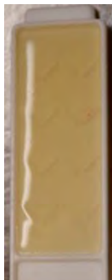
Baseline measurement with 100% biocide (under 1,000 CFU)
