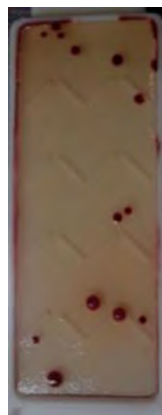
After 1.5 months with 50% less biocide (between 1,000 to 5,000 CFU)
